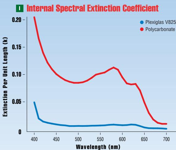
**I** Internal Spectral Extinction is a useful property for comparing the light transmitting efficiency of polymeric materials. It is independent of length and is a function of the material alone. A high extinction coefficient equates to high absorption or poor light transmission. Internal absorption can be estimated from the extinction coefficient (k) using the following relationship:
