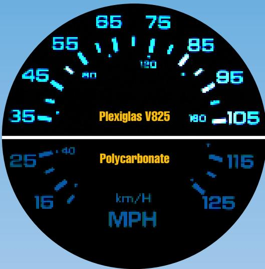
The composite photograph to the left illustrates the visual performance difference in identically illuminated subdials molded from Plexiglas V825, and polycarbonate. The lower light transmission of polycarbonate results in a reduced illumination level relative to the level achieved with Plexiglas V825.
